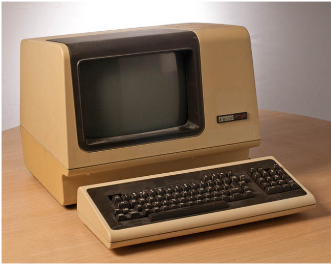
Figure 3: The VT100 Terminal that controlled Therac-25 [10]
